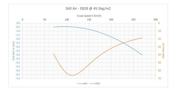
This sink and glide ratio polar seem to be a bit optimistic at low speeds (max LD 65.5), however, I think it is realistic in the speed range that matters for this flight (150km/h – 250km/h IAS).
